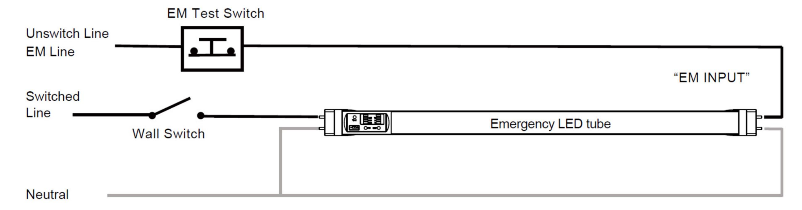
• EMERGENCY LED TUEB LAMP ALONG WITH STANDARD DOUBLE END LED TUBE LAMP WIRING
