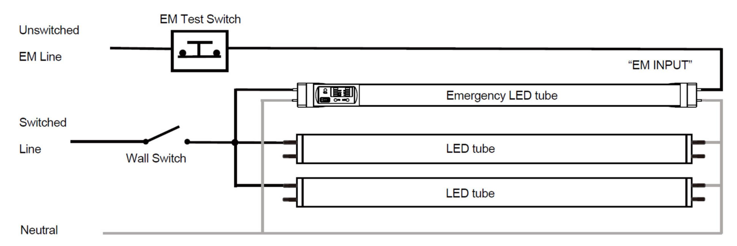
• EMERGENCY LED TUEB LAMP ALONG WITH STANDARD SINGLE END LED TUBE LAMP WIRING
